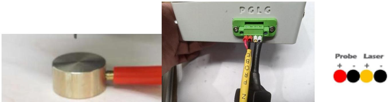
The Z probe consists of a 15mm high aluminium puck, connected with a red banana plug with a black alligator clip. Connect the red and black wire to the controller box which will have labelled either PGLG or a coloured label. The set up of the Z probe will occur during set up of Easel or gSender.
