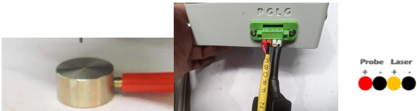
The Z probe consists of a 15mm high aluminium puck, connected with a red banana plug with a black alligator clip. Connect the red and black wire to the controller box which will have labelled either PGLG or a coloured label. The set up of the Z probe will occur during set up of Easel or gSender.
